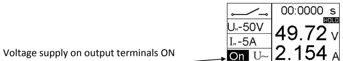
6.18 Turn the voltage and current regulator knob 10 (fig.3) to set the required voltage value, using display data.
